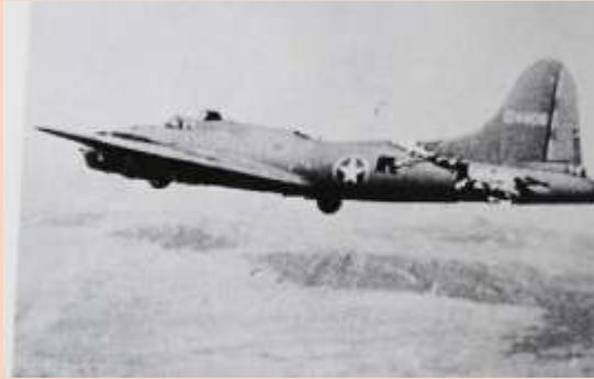
vertical fin and the rudder had been damaged, the fuselage had been cut almost completely through connected only at two small parts of the frame and the radios, electrical and oxygen systems were damaged. There was also a hole in the top that was over 16 feet long and 4 feet wide at its widest and the split in the fuselage went all the way to the top gunners turret.
